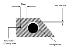
A temperature control is indispensable. We recommend that the temperature measuring point is located at a distance of less than 15 mm to the cartridge heater.
